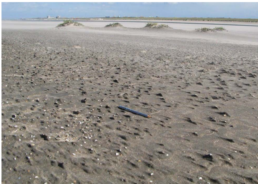
Fig. 6. Aeolian erosion marks developing on the surface of the Sand Motor mega nourishment (see pencil for scale) on October 7, 2014. Wind is blowing from the right.
