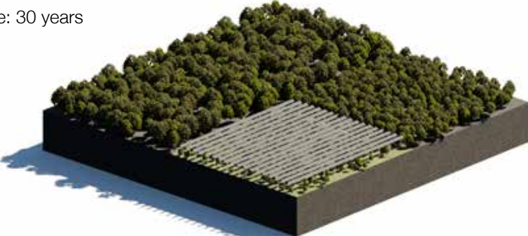
Figure 26. FV principle. Plant trees under PV-system (a), let young forest develop (b), move the PV-system as forest grows high (c), repeat until PV-panel lifetime is reached (d).
