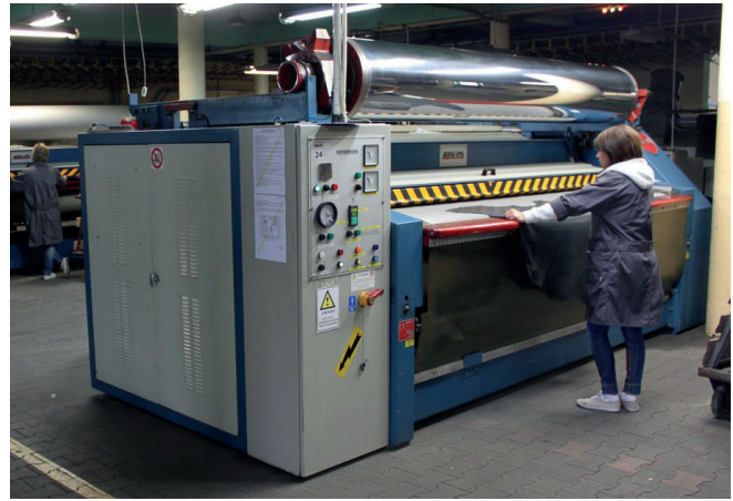
Figure 87. Rotary ironing machine, adjustable pressure
