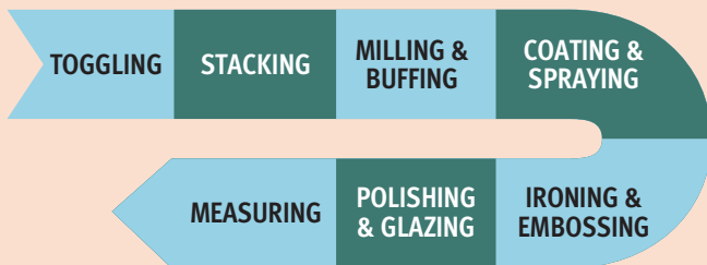
Figure 74. One of many variations of operations in preparation of wet blue for dry finishing
