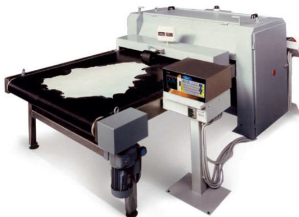
Figure 51. Electronic area measuring machine for leathers at pickled or wet blue stage
