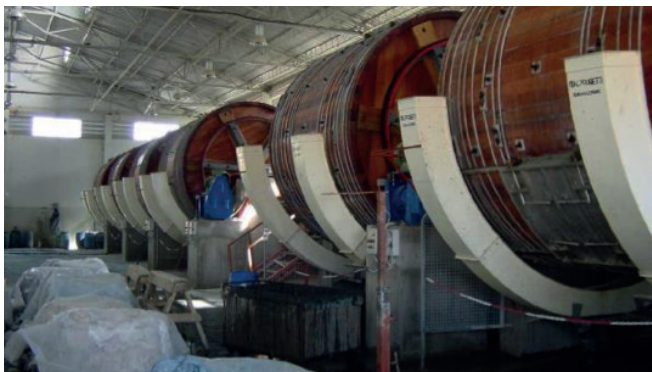
Figure 30. Hair-save system with rotary drum filter and collecting pit
