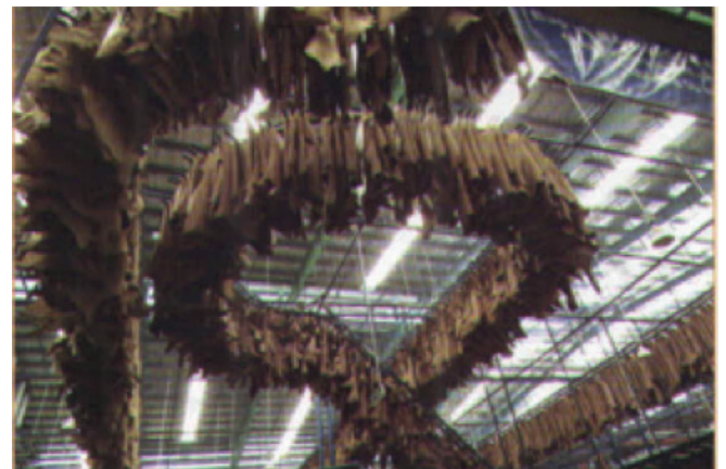
Figure 71. Tension-free drying using overhead conveyer in the tannery Saigon Tan Tec
