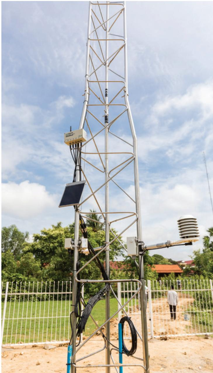
Automatic weather station installed under the project in 2018.
