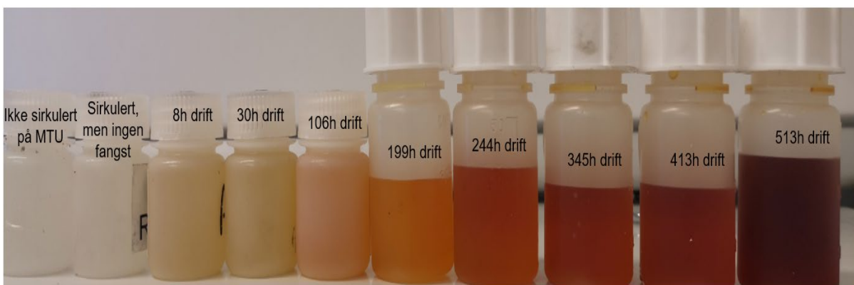
Figure 7: MEA solvent colour as a function of operating hours in the Preem CCS MTU campaign. Text in Norwegian ('drift' = 'operation')
