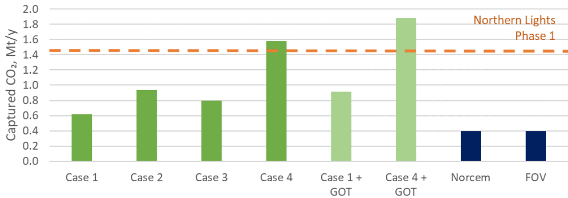
Figure 18 Potential amounts of CO 2 that could be captured in the different Preem CCS project cases compared to amounts to be captured in the Norcem and Fortum Oslo Varme (FOV) plants (Longship Project).
