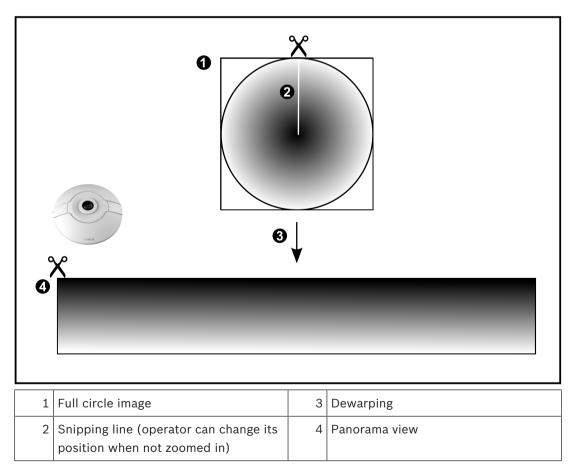
The following figure illustrates the dewarping of a 180° camera which is floor- or ceiling mounted.
