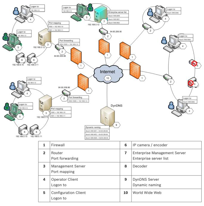
The following image shows an example of remote access from private network with Enterprise System to remote BVMS systems:
