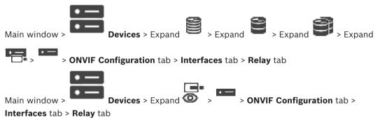
The physical idle state of a relay output can be configured by setting the idle state to **open** or **closed** (inversion of the relay behavior).
