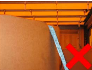
Figure 34. Example of a damaged reel edge
