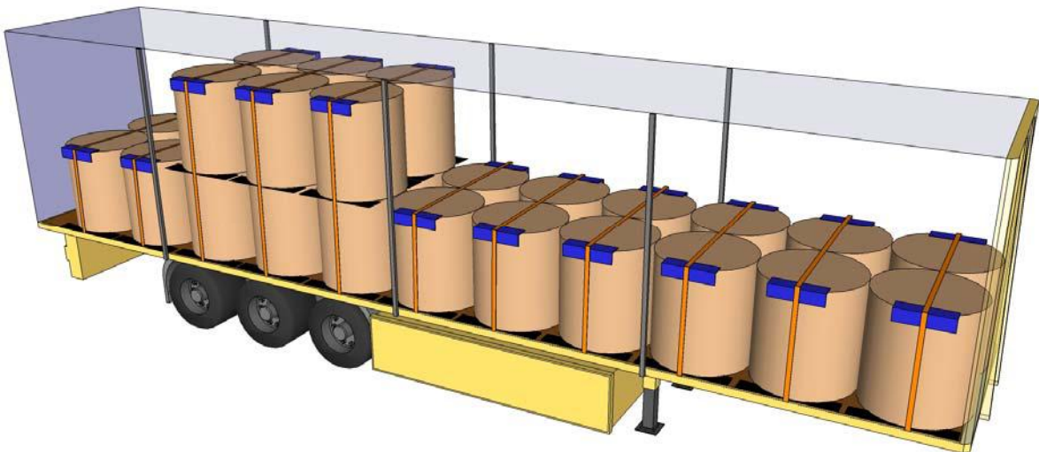
Figure 46. Curtainsider with headboard and rear wall, with rubber put underneath the reels
