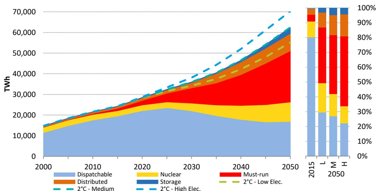
Note: Dispatchable refers to all thermal plants (including biomass and geothermal) and CSP with energy storage. Must-run refers to solar PV, CSP without storage, wind, hydro run-of-river and ocean; Distributed refers to small units of PV, CHP, fuel cells and small hydro. Storage consists of battery, compressed air, hydro lake and pumped storage and vehicle-to-grid.
