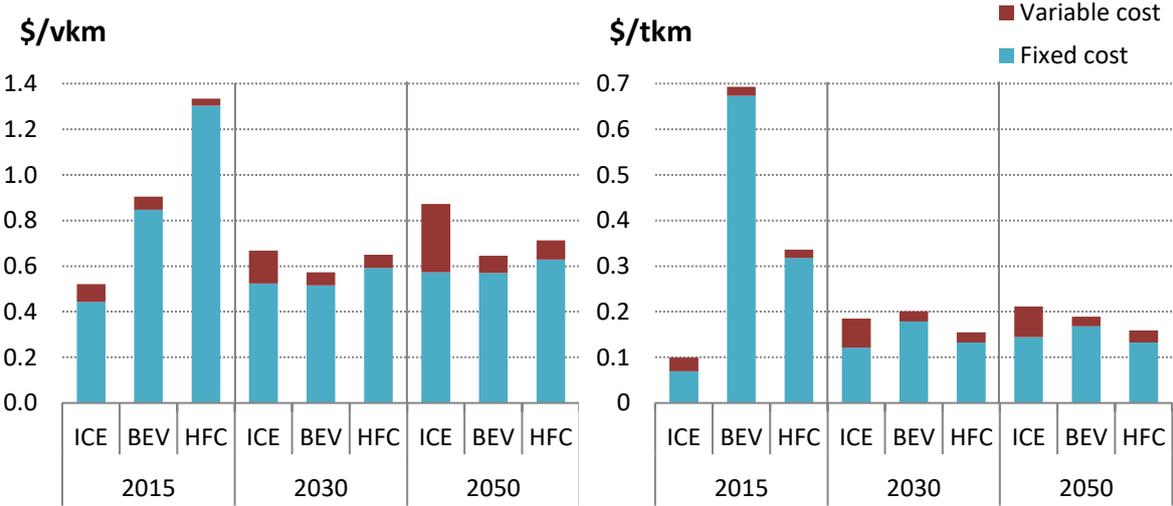
Note: Costs in real USD (2015) include the purchase cost of the vehicle, amortised over its lifetime (typically 12 years) with a discount rate (12% for LDVs, 9% for HDVs), and fuel costs (for a given year, adjusted for powertrain and vehicle efficiency, all taxes included), over the vehicle's use in a year (region-dependent).
