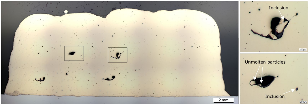
Fig. 6: Polished sections of 10-layer cube from sieved grinding material.
