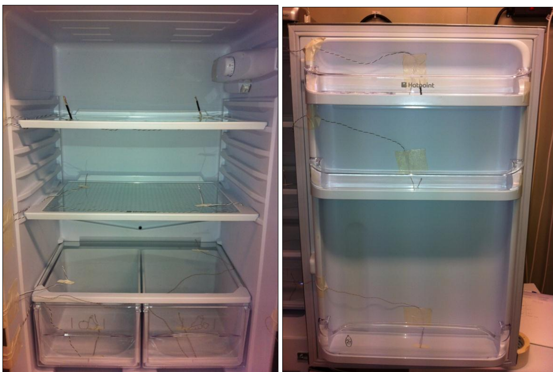
Figure 11 Photographs showing thermocouple positioning for air temperature measurement
