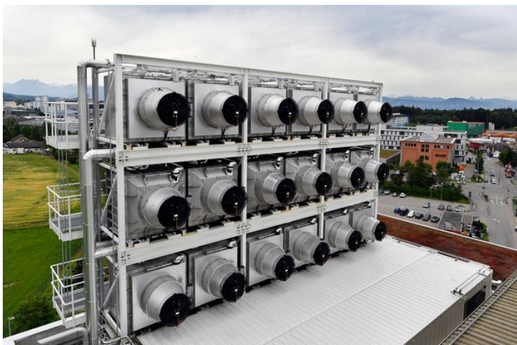
Figure 14 Climeworks pilot DAC facility located in Hinwil, Switzerland, with 18 module units each separating \sim 50\text{tCO}_2/\text{yr} . [figure copyright Climeworks].
