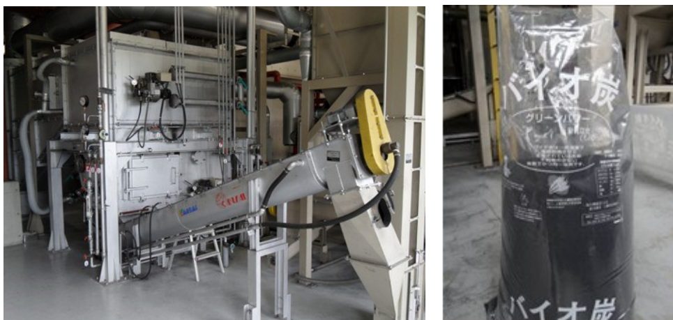
Figure 7 – a) small-scale (1.5t/day) rice husk pyrolysis unit developed by Kansai Corporation, in Shiga, Japan, b) 100L (30kg) bag of rice husk biochar prepared for sale.
