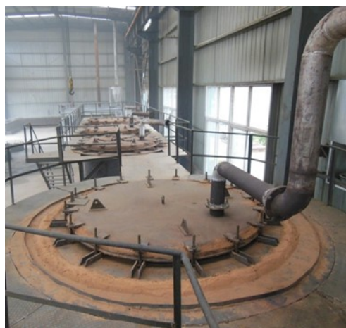
Figure 8 – A poly-generation plant in Wuhan, China, based on a simple and well-established retort technology.
