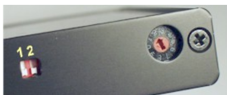
Figure 4 DIP switches and rotary switch.
