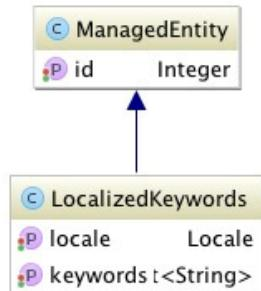
Figure 11 LocalizedKeywords UML class diagram
