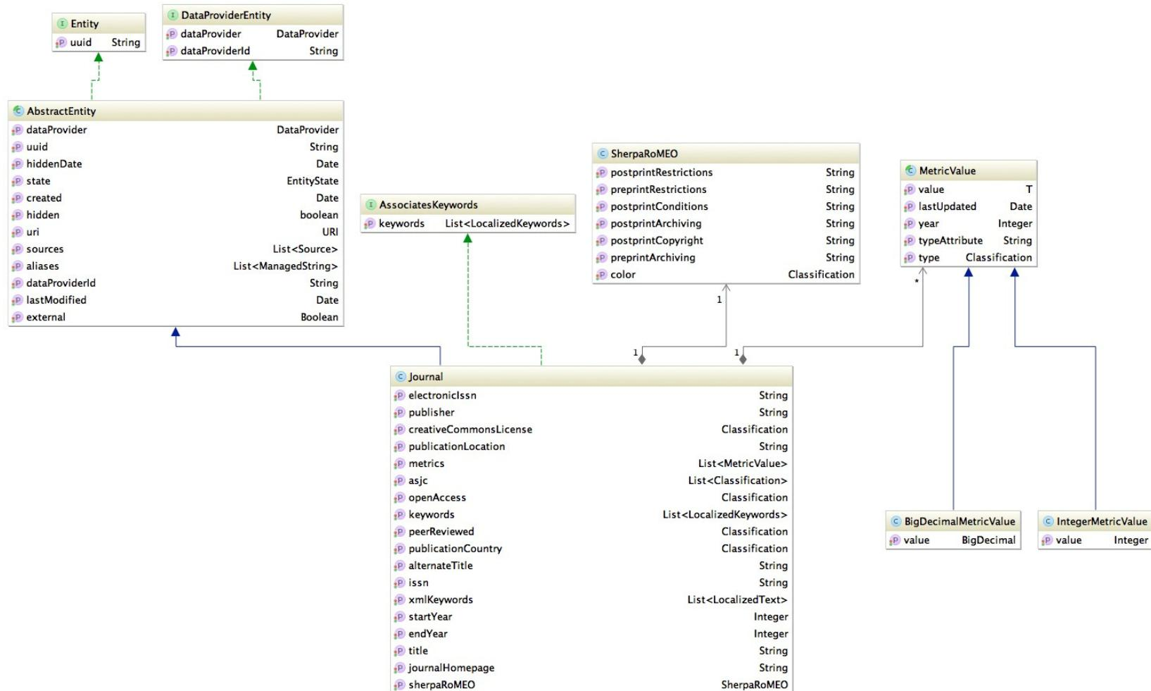
Figure 5 Journal UML class diagram
