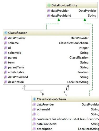
**Figure 7 Classification scheme & classification UML class diagram**
