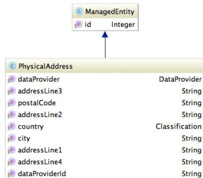
Figure 8 Physical address UML class diagram
