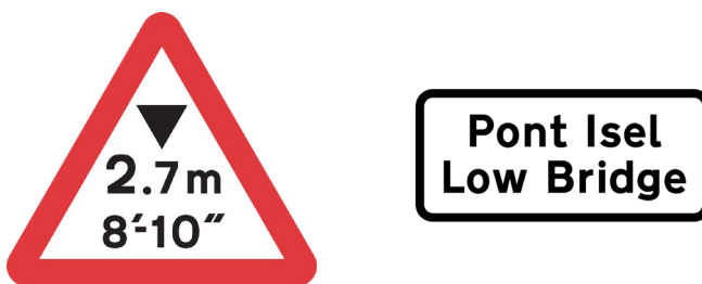
Figure 9.12 – Low headroom signage (diagram 530A) and associated sign plate example
