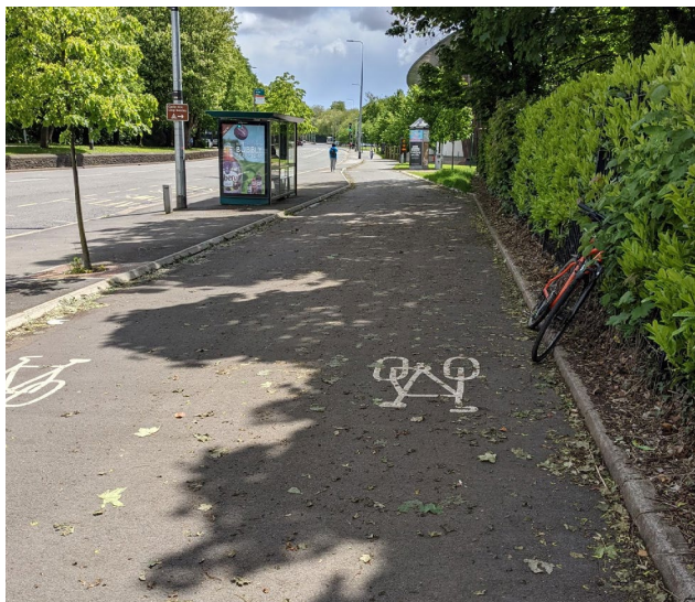
Figure 11.21 – Bus stop bypass
