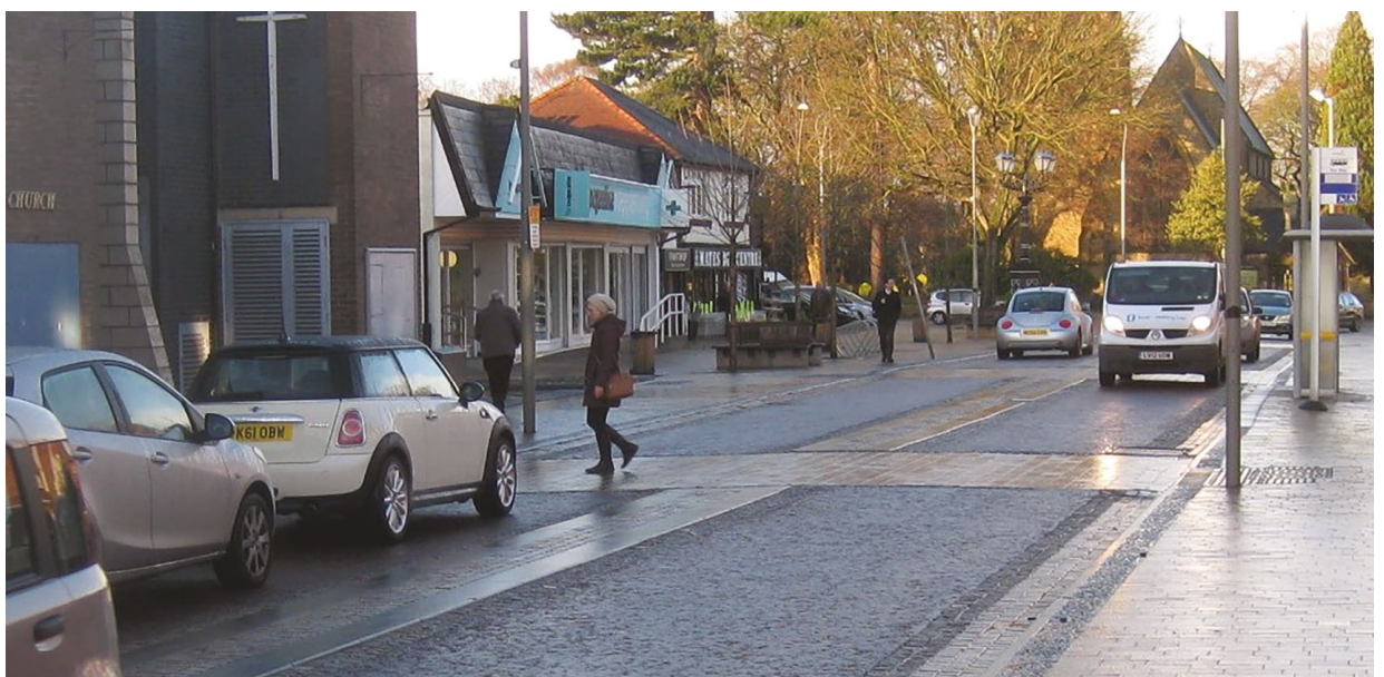
Figure 12.7 – Informal median strip, Poynton, Cheshire
