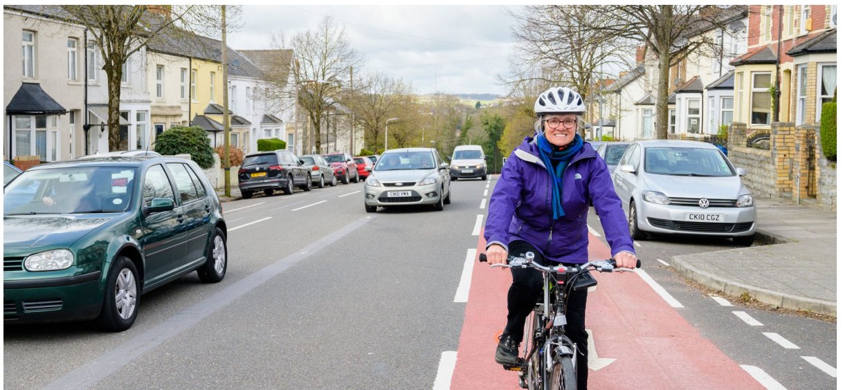
Figure 11.13 – Centre line removal to allow advisory cycle lanes, Penarth
