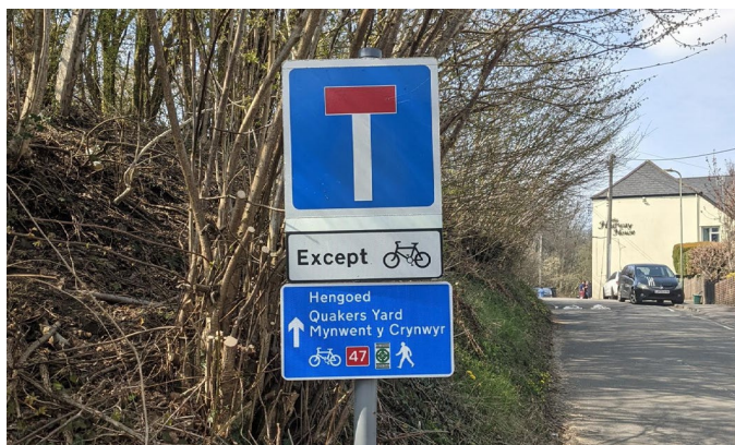
Figure 14.9 – No through road with except cycles plate and directional signage (Except should be bilingual)
