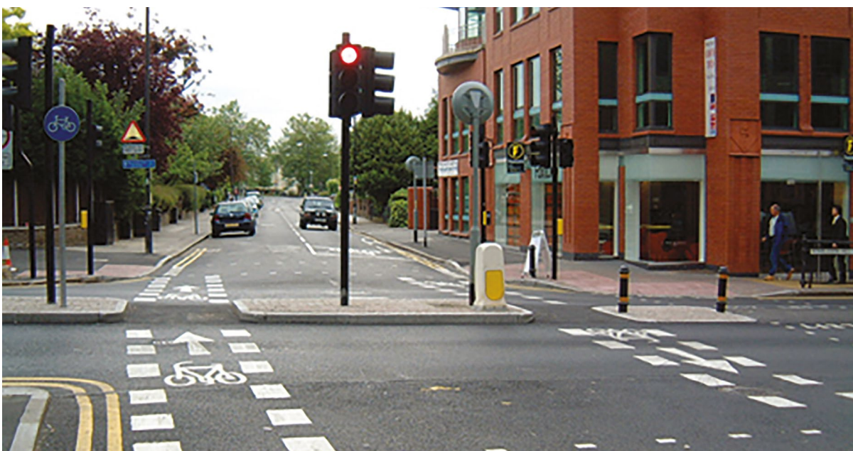
Figure 12.17 – Elephant footprint markings through junction
