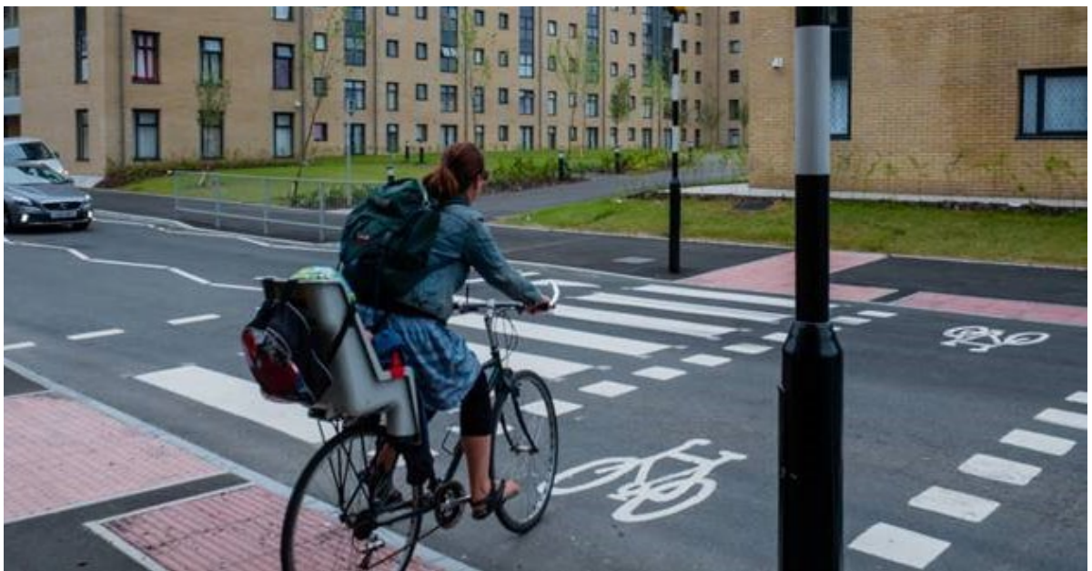
Figure 12.9 – Parallel crossing for pedestrians and cyclists, Cardiff
