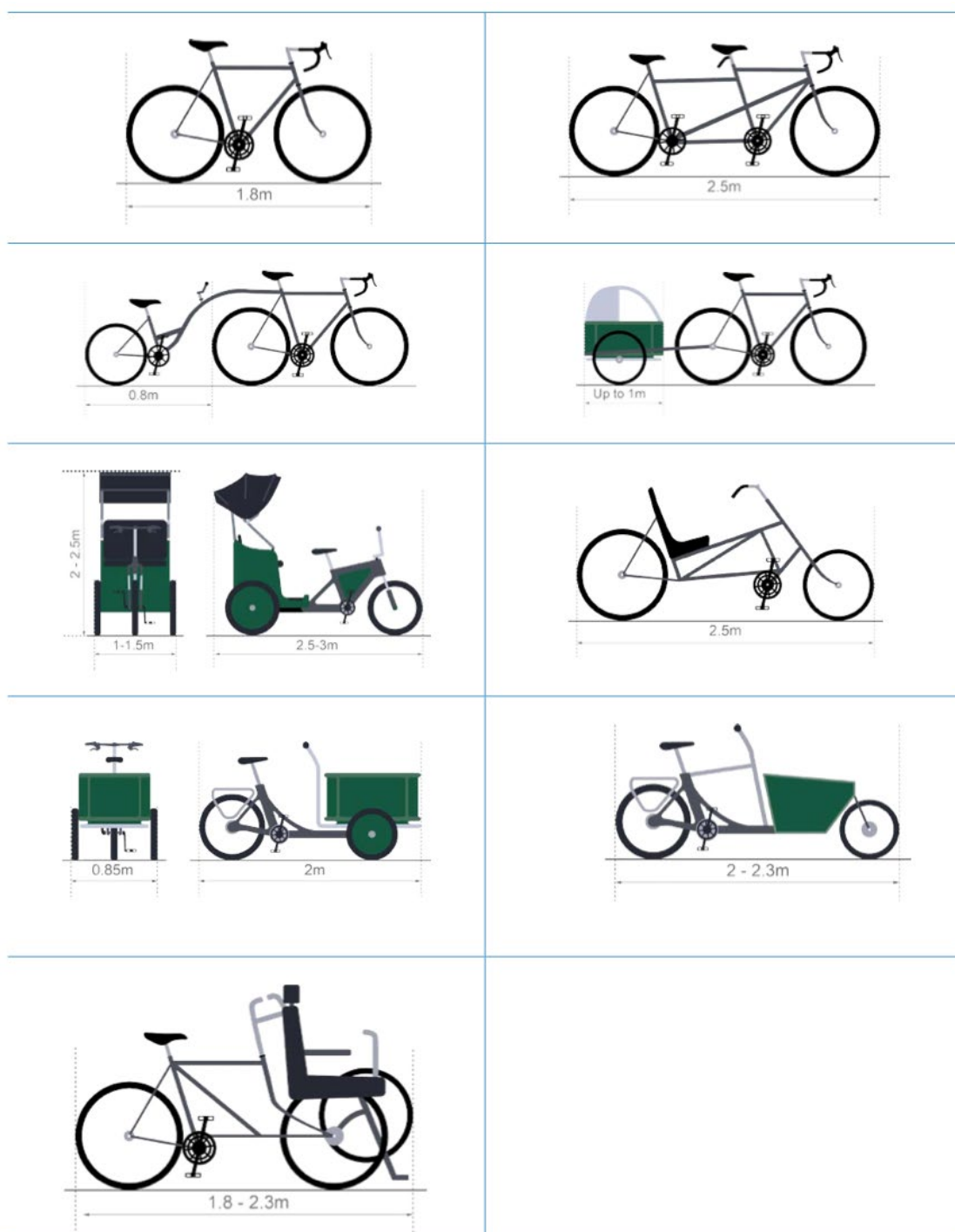
Figure 9.11 – Types of cycle with dimensions
