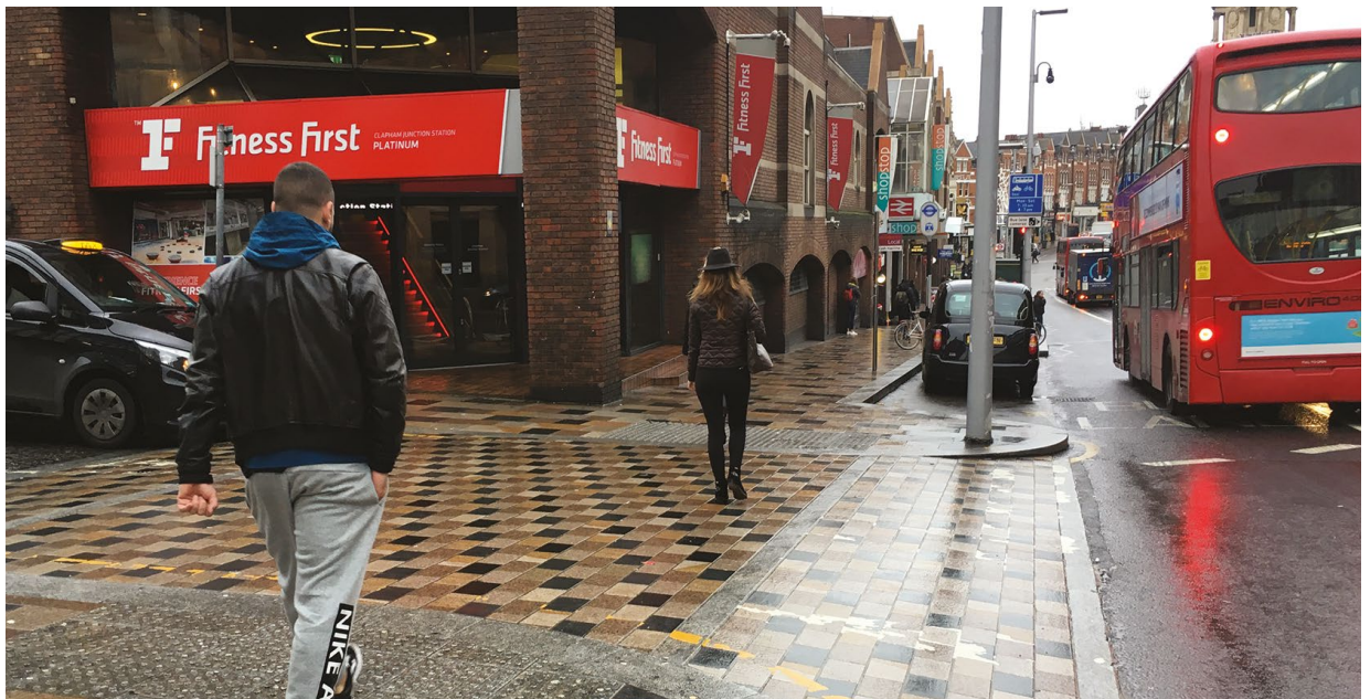
Figure 12.5 – Semi blended footway at side road with kerb line and tactiles retained, Clapham
