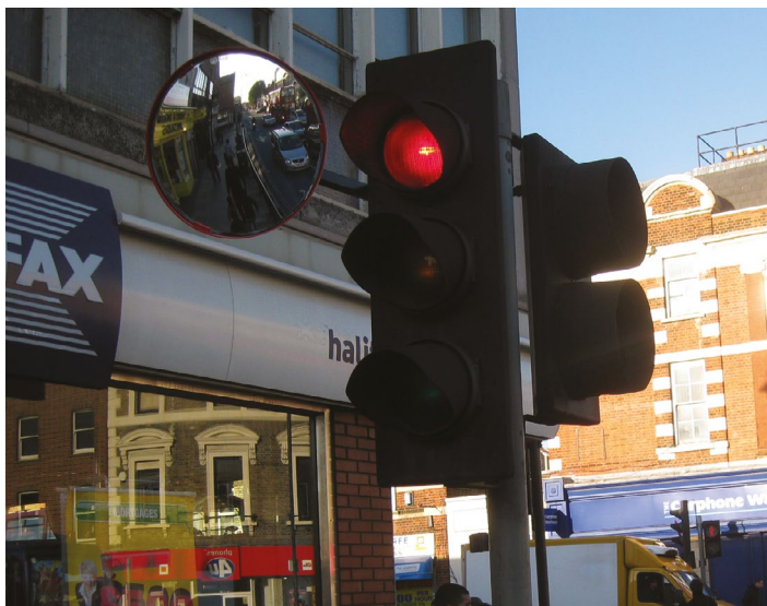
Figure 12.20 – Trixi mirror on cycle superhighway 7, London
