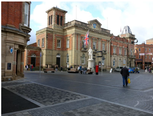
Exchange Square, Kidderminster. Blended crossing (with tactiles) on approach to a junction/public square with no designated priorities.
