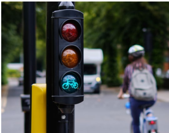
Figure 12.10 – Early start low level cycle specific light, Cardiff
