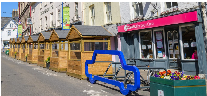
Figure 14.7 – Parallel parking bay provision replaced with cycle parking and public seating areas
