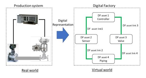
Figure 5 – Simple Digital Factory example
