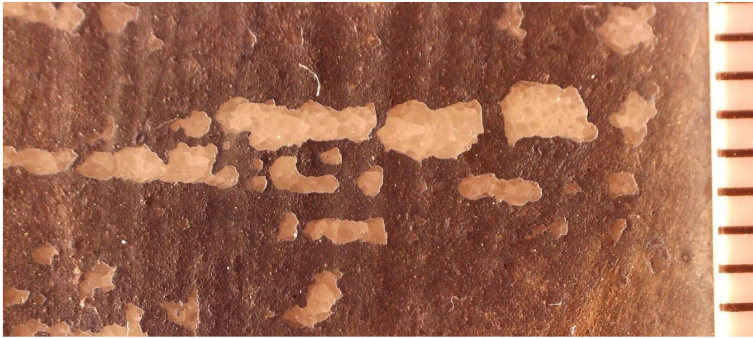
Figure 16. Linear abrasions resulting in paint detachment. The vertical lighter and darker ridges and furrows are paint brush strokes. Again, the false colouring is the result of side lighting. Scale is mm.
