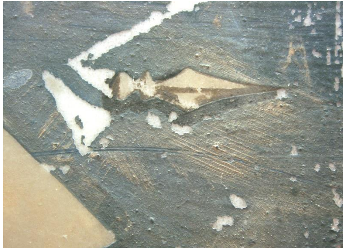
Figure 14. An ochre coloured surface deposit that seeming has attempted to be wiped away when wet. This striated deposit stops abruptly at the edges of peeled paint and spearheads and does not continue onto either.
