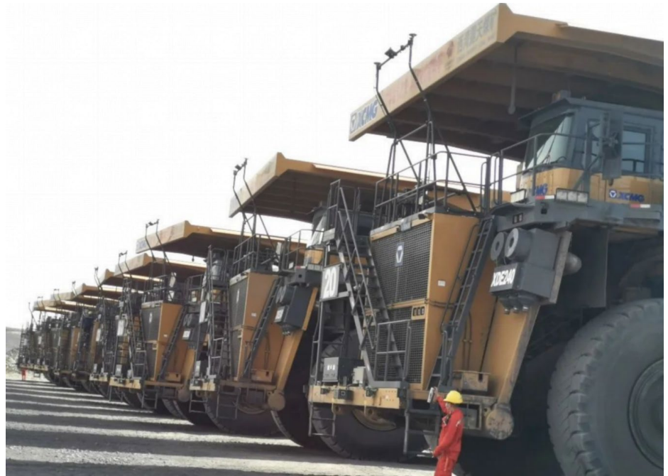
Unmanned Mining Trucks Synergized with Auxiliary Vehicles in Loading, Transportation, and Unloading at Xiwan Surface Mine
